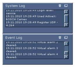
The **System Log** field contains information about the operating status of the VOT-320 and the connection. You can save these messages automatically in a file (see *Section 5.14 Advanced Mode: LIVEPAGE Functions, page 38*).
